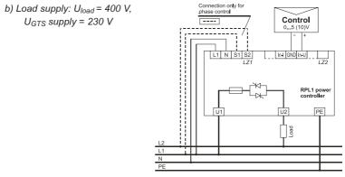
Fig. 4.9. Connection diagramm of load in single-phase system.
