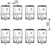
Fig. 4.2. Intervals between power controllers
