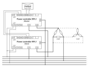
Fig. 4.10 Connection diagram of a load in three-phase system
