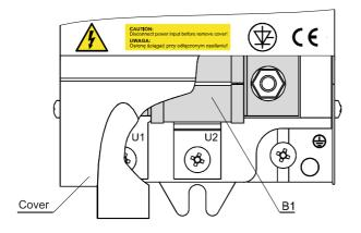
Fig. 4.8. View of the high-current power controller circuit
