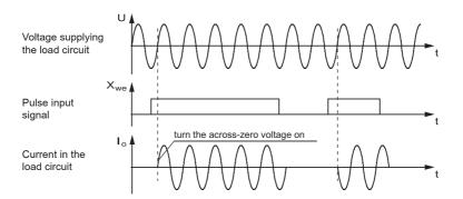
Fig. 5.1. Control of on-off type, runs of occurring signals (for resistive load).
