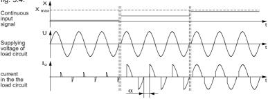
Fig. 5.4. Phase control, runs of occurring signals
