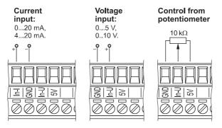
Fig. 4.5. Connection of control signals
